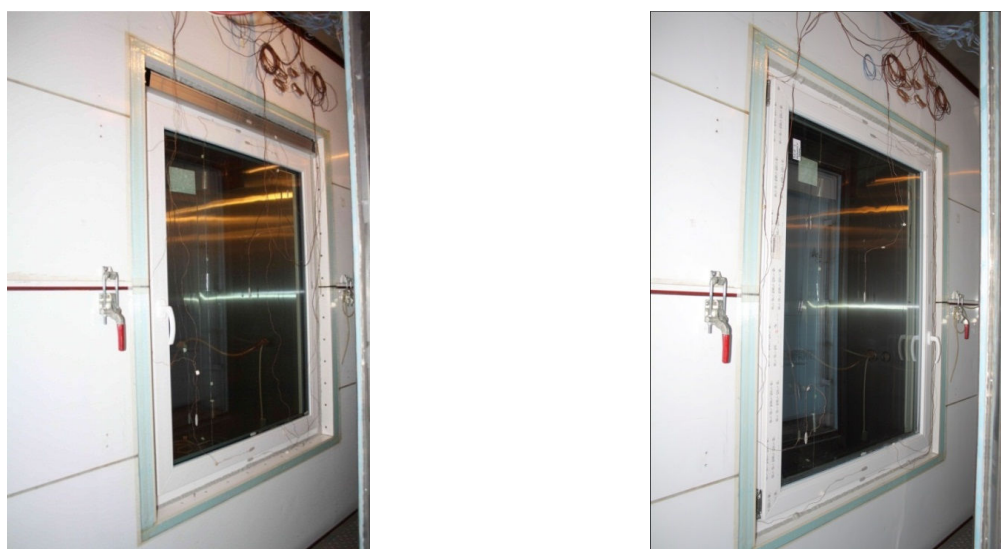
Figure 11. A view from the interior (from the warm chamber) to the Rehau Geneo PHZ window mounted in the mask panel of the chamber, on the left with the installed ventilation unit and on the right window itself without the ventilation unit.
