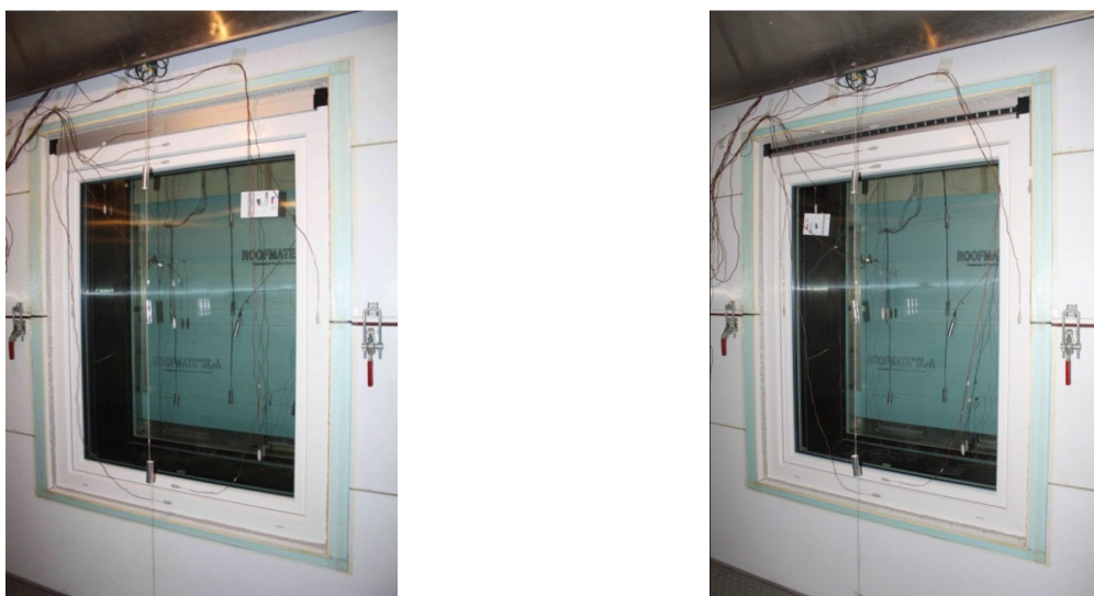
Figure 10. View from the outside (from the cold chamber) to the Rehau Geneo PHZ window with an installed ventilation unit mounted in the mask panel of the climate chamber, the Renson Invisivent EVO AKD Max on the left and Renson Invisivent EVO AK Basic on the right.
