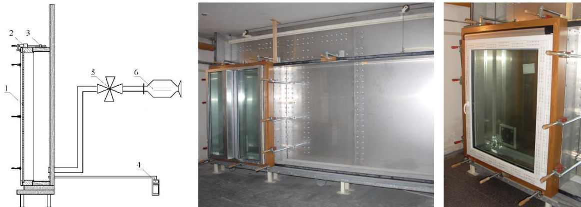
Figure 5. Scheme and view of large pressure chamber and view of the window with inlet vent flap installed to the masking panels in a large pressure chamber. 1 – test sample, 2 – mounting frame, 3 – large pressure chamber, 4 – barometer, 5 – four-way valve, 6 – fan.
