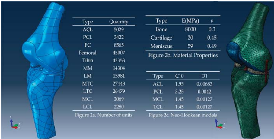
Figure 2. Mesh generation and material properties of knee models. The right figure represents assembled knee model. In the left figure, different colors define the different material properties. ACL: anterior cruciate ligament; PCL: posterior cruciate ligament; FC: femoral cartilage; MM: medial meniscus; LM: lateral meniscus; MTC: medial tibial cartilage; LTC: lateral tibial cartilage; MCL: medial collateral ligament; LCL: lateral collateral ligament.
