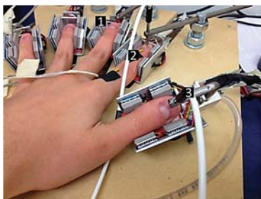
Figure 2. The iGlove-1 -controlled cooling device for the left hand. (1) Peltier cooling elements; (2) NTC temperature sensor to measure the finger skin temperature; (3) one probe of the blood flow Laser Doppler meter.
