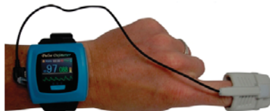
Figure 1. The CMS50FW wearable oxygen saturation (SpO 2 ) and pulse rate device with wireless communication for real-time vital-sign monitoring.
