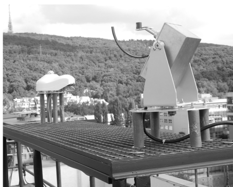
Figure 1. View on the pyranometers at the platform.
