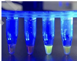
Figure 3. Readout signal of COVID-19 samples with GeneFinder dye under blue light. Left are negative controls and right are positive samples.[14] (Reprinted from ref. 14)
