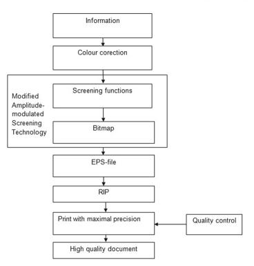
Fig. 1. Block diagram of screening technology
