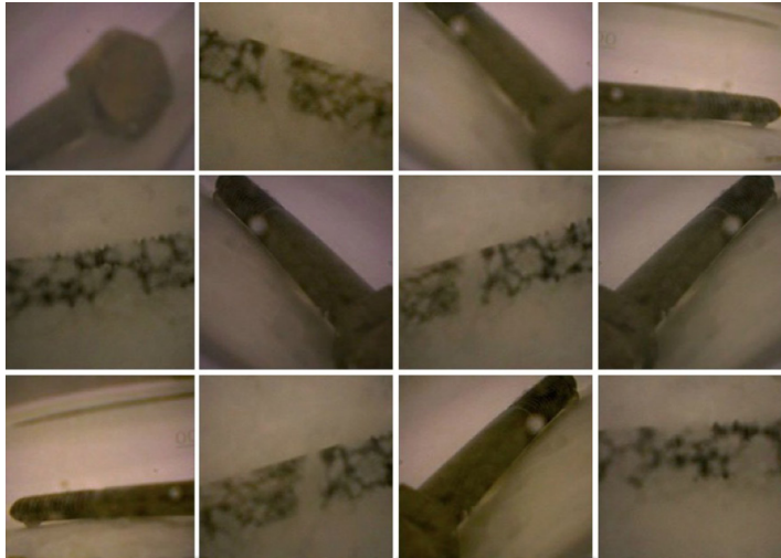
Figure 10.23: In the presence of a rusty bolt, 'protopearl'-producing DEPP droplets produced a significant flocculent precipitate, which was not confined to the oil/water interface. Photographs and collage, Rachel Armstrong, February 2009.
