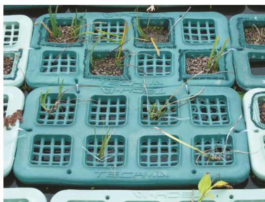
Figure 4. Particular of two TECH-IA® elements in which the plants were set with (above) or without (below) the substrate of expanded clay.
