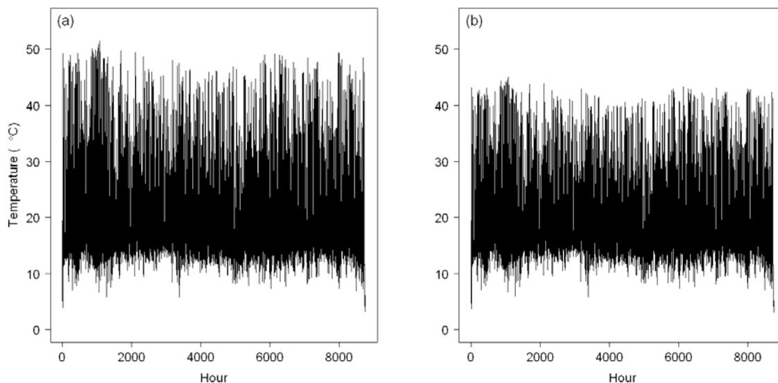
Fig. 2. Yearly simulated temperature profiles of greenhouses covered with (a) glass and (b) polyethylene under the Bogota plateau climate. The simulations in both cases were carried out for fully closed empty greenhouses.
