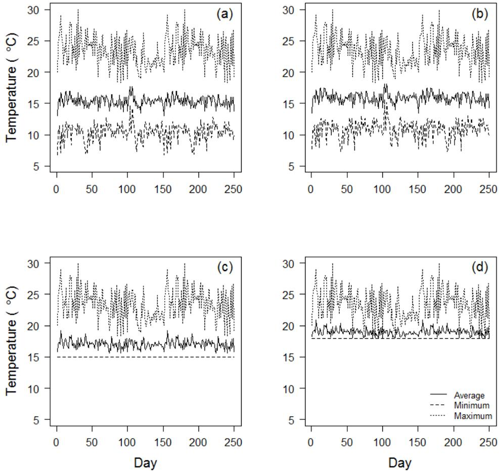
Fig. 3. Daily temperature profiles of the climatization alternatives (current greenhouse design, (a) addition of thermal screen (b) and addition of heating with set-points at 15°C (c) and 18°C (d)) used to evaluate the growth of a 250-day tomato cropping cycle in the Bogota plateau.
