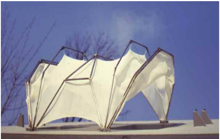
Exercises on the convertible roofs carried out under Frei Otto's supervision, Warmbronn 1969 the sewing experience I gained in my father's tailor shop was put to good use
