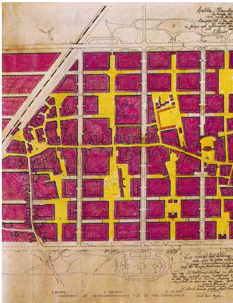
Location plan of the urban expansion of Aalter; the pedestrian zones are marked yellow and dock vertically onto the historical one-street village. These represent the heart of each new district. The urban space components are expressed here for the first time.
