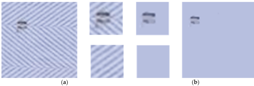
Figure 4. Smoothed fabric defect image using L0 gradient minimization (LGM). (a) Fabric defect image; (b) Smoothed fabric defect image.
